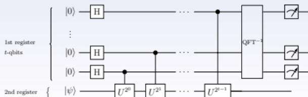
Figure 1: Quantum phase estimation by a quantum circuit acting on the initial state  $|0\rangle^{\otimes t} \otimes |\psi\rangle$ : H-boxes are Hadamard gates,  $U^{2^i}$ -boxes stand for CU-operators,  $i = 0, \dots, t-1$ ,  $QFT^{-1}$  for the inverse quantum Fourier transform, and the last stage involves a measurement on the first register.
