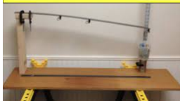
Cantilever beam for measuring material stiffness
