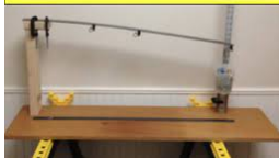
Cantilever beam for measuring material stiffness
