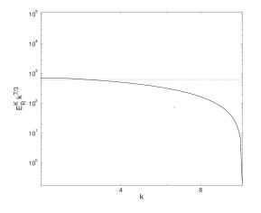
Figure 3: Normalized, time-averaged and smoothed spectrum of the residual energy, multiplied by  $k^{7/3}$ , for the first case.
